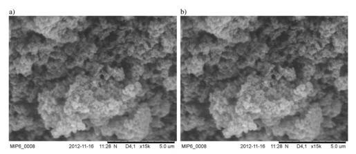
Fig. 3. The SEM image of BPA-imprinted polymer (MIP 6, prepared with AA in CH<sub>3</sub>CN). a) MISPE without washing; b) MISPE with washing step with toluene. SEM image magnified 10,000-fold
