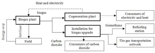
Fig. 3. Material and energy flows of biogas plant
