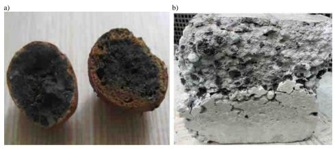
Fig. 1. Samples used for examinations: a) lightweight aggregate with sewage sludge burnt at a temperature of 1150°C - fracture, b) sample of lightweight-aggregate concrete with sewage sludge after 30 freezing cycles
