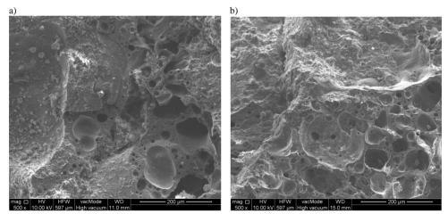
Fig. 5. Hydrophobized structure lightweight-concrete (500x): a) water-soluble preparation - A1, b) organic solvent-ased methylosilicone resin - A2
