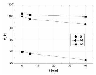
Fig. 3. Water-contact angles in lightweight-aggregate concrete modified with sewage sludge
