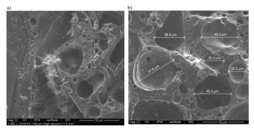
Fig. 4. Scanning microscope images of the structure: a) lightweight aggregate-concrete, b) lightweight aggregates with measurement of pore sizes
