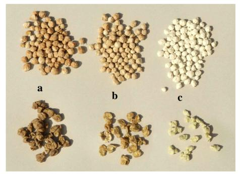
Fig. 5. Particles of fertilizers covered by films of the composites of PVA with rapeseed cake (a), horn meal (b) and phosphogypsum (c) before (above) and after keeping in water for three hours (below)
