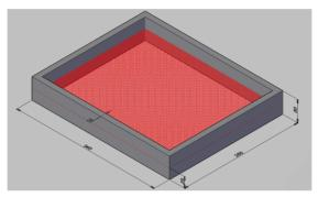
Fig. 2. Image of the wooden frame
