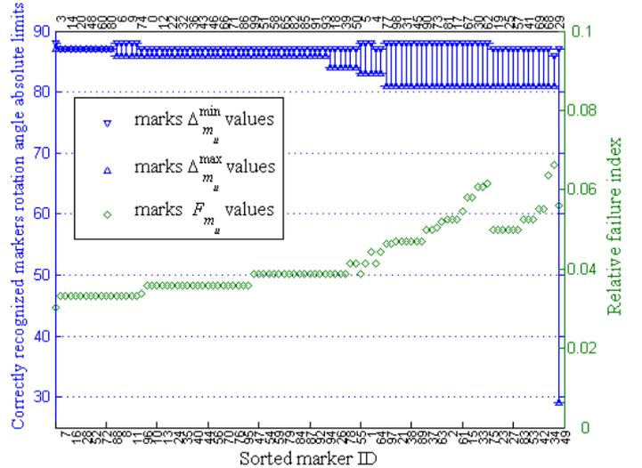
Fig. 10. Marker recognition results sorted using three-fold criteria: (4a), (5), and (8). Note: marker IDs are shown pair wise at the bottom and the top of axis; relative failure index  $F_m$  values are indicated at the right side of axis.
