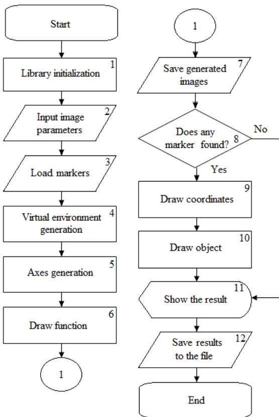
Fig. 4. Flowchart of augmented reality system implementation.
