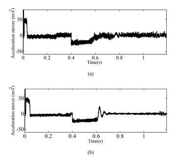
Fig. 6. Acceleration of the mover (a) by using a conventional sliding mode observer (b) by using the proposed sliding mode observer.
