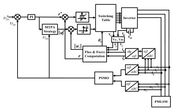
Fig. 2. Block diagram of the PMLSM sensorless control.
