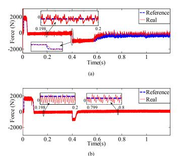
Fig. 7. The produced force of the mover (a) by using a conventional sliding mode observer (b) by using the proposed sliding mode observer.
