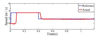
Fig. 5. Speed reference signal and speed actual of the motor by the proposed sliding mode observer.
