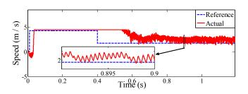
Fig. 4. Speed reference signal and actual speed of the motor by sliding mode observer.
