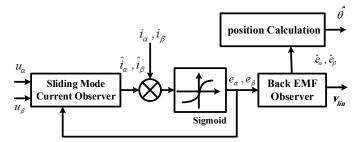
Fig. 3. Block diagram of the purposed sliding mode observer (PSMO).
