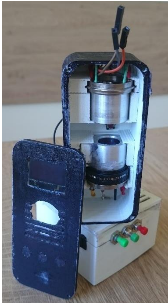
Fig. 3. The non-invasive optical glucometer prototype with the ellipsoidal reflector.
