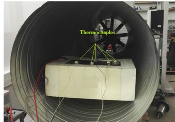
Fig. 5. Coil box inside the wind tunnel and location of the thermocouples.
