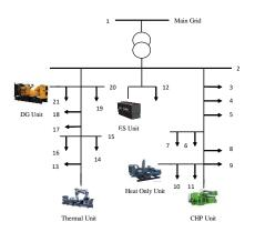
Fig. 1. Configuration of the 21-bus microgrid system.
