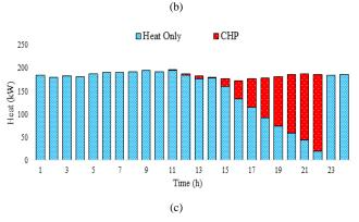
Fig. 7. Generated heat of CHP and heat only units, a) first case; b) second case; c) third case.
