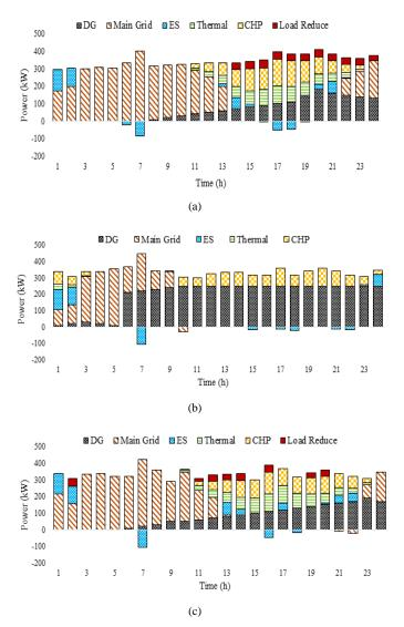
Fig. 6. Generated electrical power of units and the main grid, a) first case; b) second case; c) third case.
