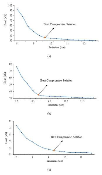
Fig. 5. The best compromise solution determined by fuzzy decision-making process in Pareto-optimal front. a) first case; b) second case; c) third case.
