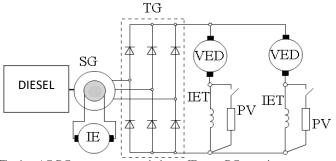
Fig. 1. AC-DC power transmission: IE - DC motion generator; SG – synchronous generator; TG – rectifier; VED – electric traction engine; IET – motion winding; PV – magnetic flux attenuator.
