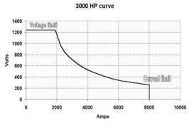
Fig. 2. Typical main generator constant power curve at "notch 8".
