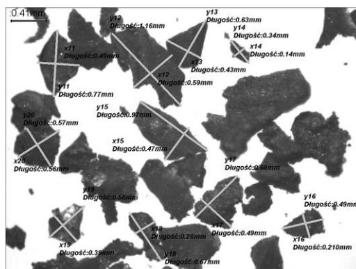
Fig. 3. Shape and size analysis of rubber granulate particles (mag.  $\times 60$ )
