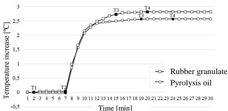
Fig. 4. Increase of water temperature during the calorimetric measurement process for rubber granulate and pyrolysis oil
