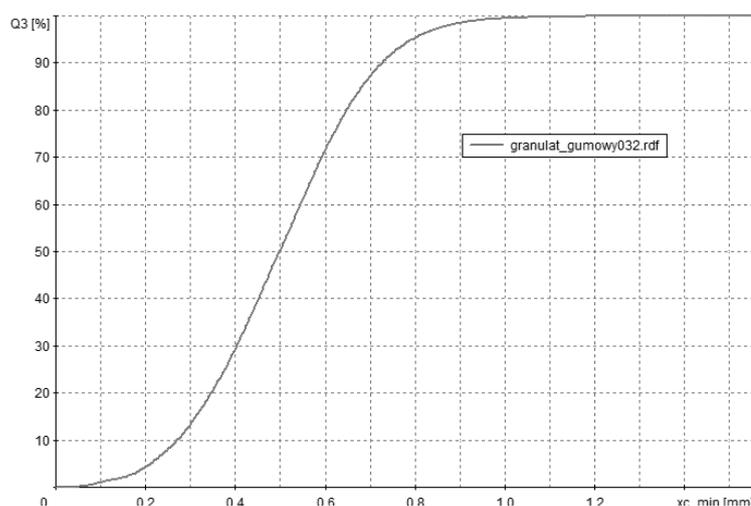
Fig. 2. Granulometric cumulative distribution of rubber granulate
