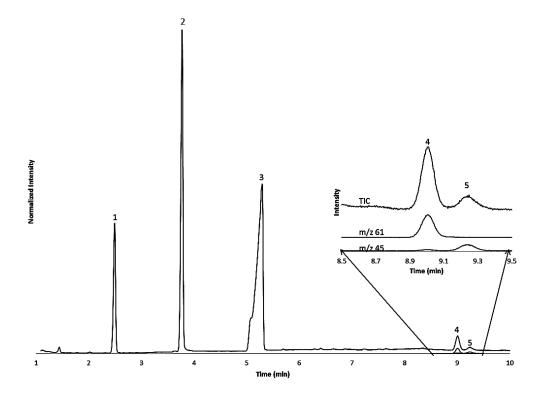
**Figure 2. Chromatogram of tobacco sample #5.** Inset demonstrates the added benefit of using MSD to ensure chromatographic separation of glycerol and triethylene glycol. Peak labels 1: propylene glycol, 2: 1,3-butanediol (IS), 3: nicotine, 4: glycerol, 5: triethylene glycol.
