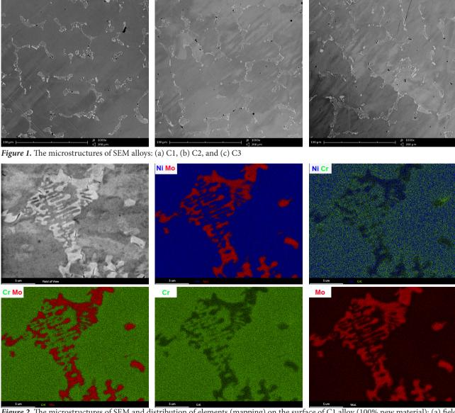
Figure 2. The microstructures of SEM and distribution of elements (mapping) on the surface of C1 alloy (100% new material): (a) field of view, (b) Ni and Mo, (c) Ni and Cr, (d) Cr and Mo, (e) Cr, (f) Mo
