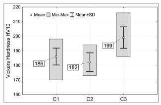
*Figure 3.* A comparison of the Vickers hardness of alloys studied groups Remanium CS + (N = 40)
