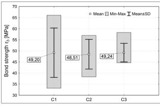
Figure 4. Summary of results of bond strength of metal-ceramic Remanium CS + alloys involving materials after recasting – results of three-point bending test conducted according to ISO 9693 ( N = 9)
