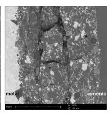
Figure 5. Microscopic SEM image of cross sections of metal-ceramics after adhesion testing for: (a) C1 castings made in 100% from the new factory material, (b) C2 castings made with 50% addition of recast material – cast once, (C) C3 castings made with 50% addition of recast material – cast twice.
