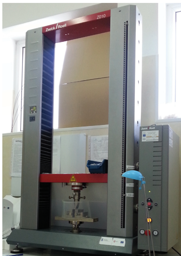
Figure 2. Testing device - flexural strenght
