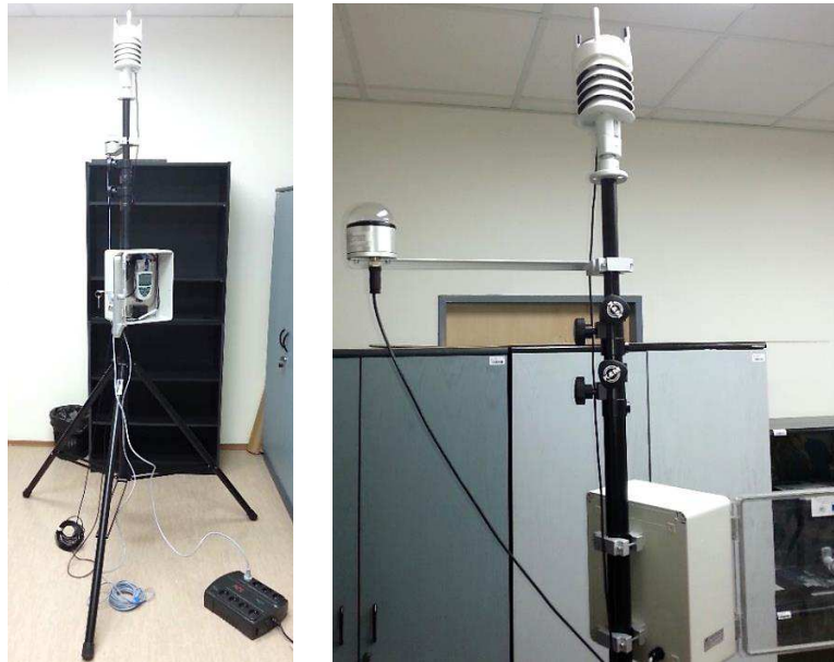
Fig. 1: Test measurement before installation into the exterior (Ahlborn Meteo FMA520).
