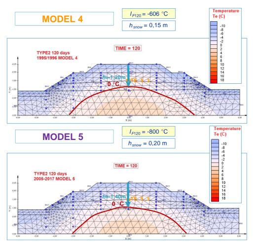
Fig. 7: Visualization of analysed results of modelling MODEL 4 and 5 - unsatisfactory.
