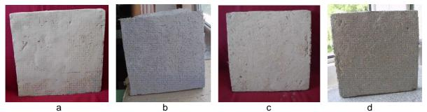
Fig. 1: General view of tested samples: a) without addition of straw; b) with 0.3 wt.% straw; c) with 0.4 wt.% straw; d) with 0.5 wt.% straw.
