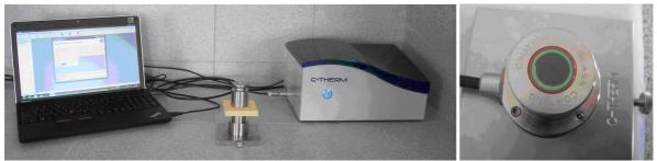
Fig. 2: TCi analyser (a) and C-Therm TCi Sensor (b).
