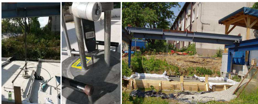
Fig. 6: Measuring system TEE (left) and view of the device examining the sag in the middle of the board (center) and view of the experimental field (right).
