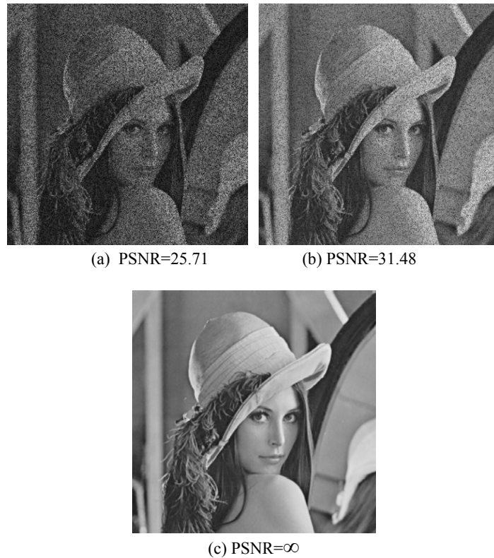
Fig. 4. Images reconstructed in the proposed (2, 4) sharing method with any (k-1) and last share
