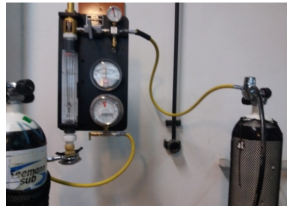
Figure no. 4. Testing the pressure regulator with Scuba Tools unit stand (Stanciu, 2018)
