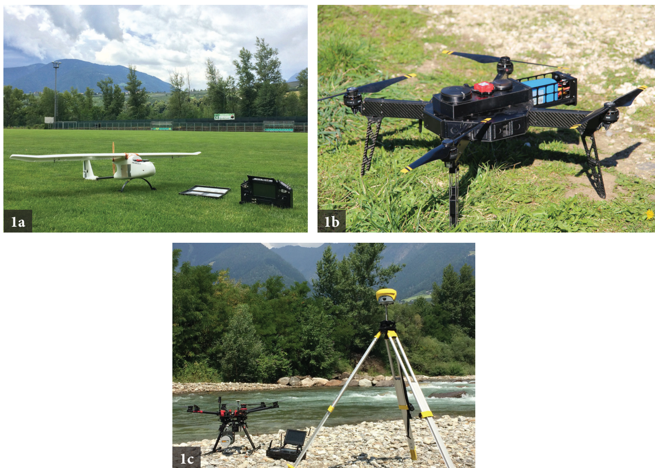
Figure 1. The three aircrafts used for the monitoring purposes: (a) AGRI-1900, (b) Q4E, (c) DJI S900 with the RTK-GNSS base for RINEX files collection. The first two solutions are two prototypes specifically developed to answer to the project's requirement, while the third is a commercial UAV, which has been modified to carry the Yellowscan Surveyor sensor.
