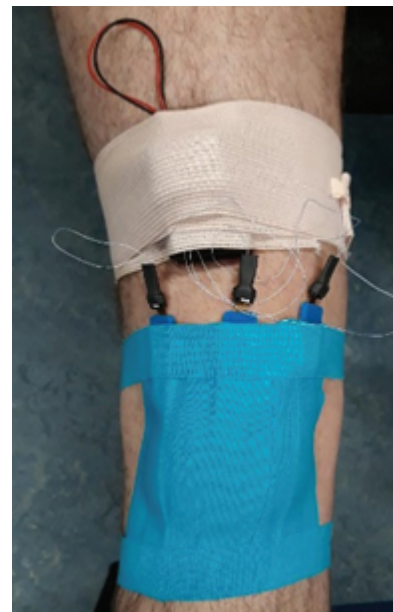
Fig. 1. Sensor placement for 3 areas and attached on the right knee by Kinesiotape with the Bluetooth communicator fixed by an elastic bandage
