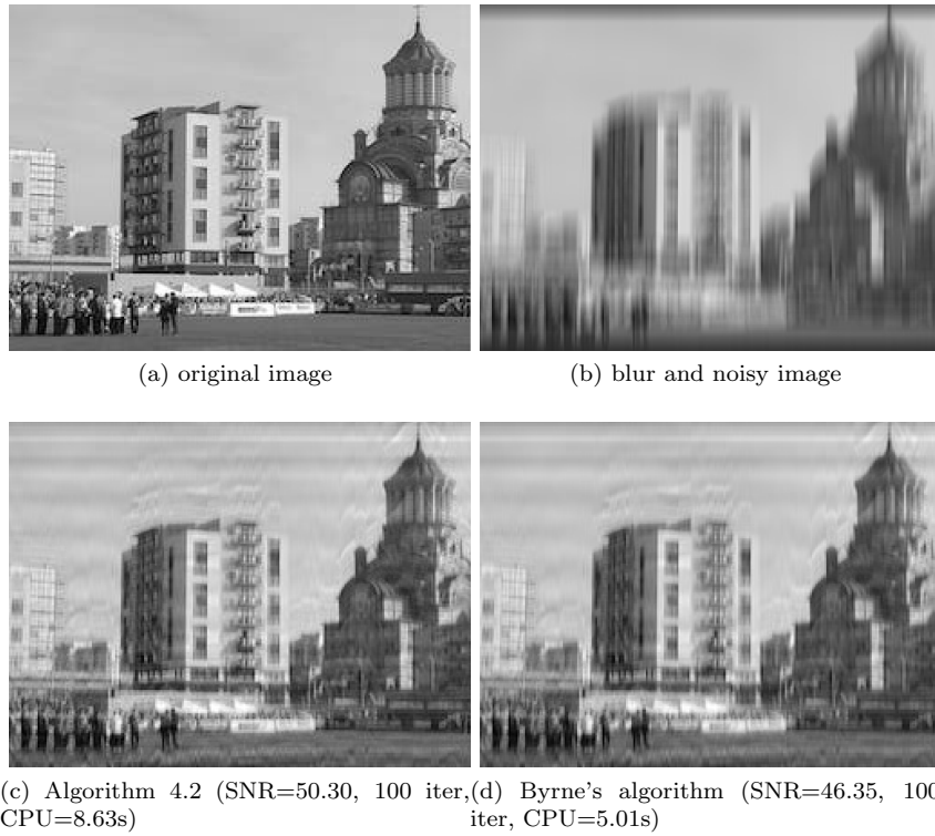
Figure 4.3: Result of restoration image size 192 \times 256 : (a) original image, (b) blur and noisy image, (c) restoration by Algorithm 4.2 and (d) restoration by Byrne' s algorithm
