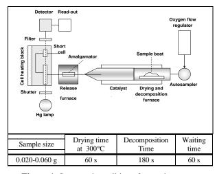
**Figure 1**. Steps and conditions for total mercury determination in fish by DMA-80
