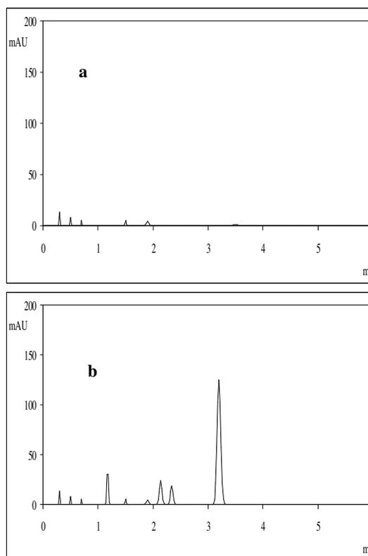
**Fig. 1.** Chromatogram of blood sample containing the blank (a) and the four benzodiazepines (b). Chromolith Performance (RP-18 100 x 4.6 mm). The mobile phase consisted of phosphate buffer (pH 2.5)/acetonitrile (65/35, v/v). The detector wavelength was 220 nm. The flow rate was maintained at 2 mL/min. The injection volume was 20  $\mu\text{L}$  and run-time 5-6 minutes.
