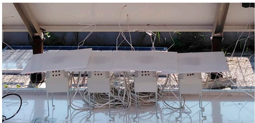
Fig. 1 Measuring system for temperature identification of PV modules
