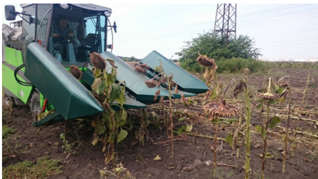
Fig. 4 Four-row header during harvesting of sunflower variety Dzhinn
