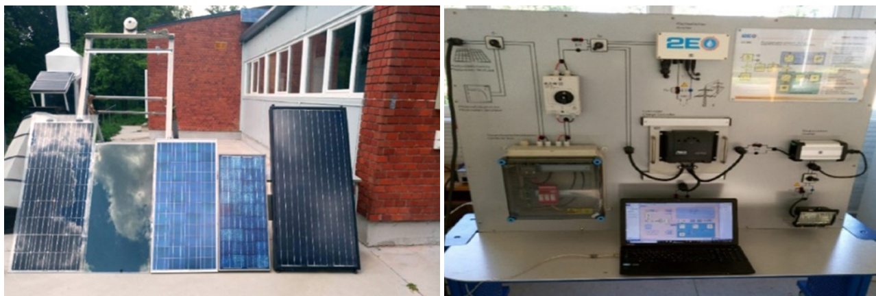
Fig. 1 PV modules and experimental setup for data collection
