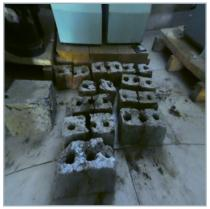
Figure 11 Crackeded bricks during M.O.R. test
