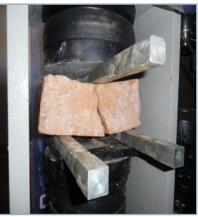
Figure 10 M.O.R. test
