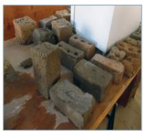
Figure 5 Termite mound brick specimens
