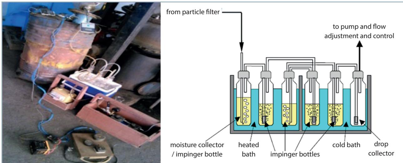
Figure 1 Schematic arrangement of sampling equipment and impinger bottles for tar collection
