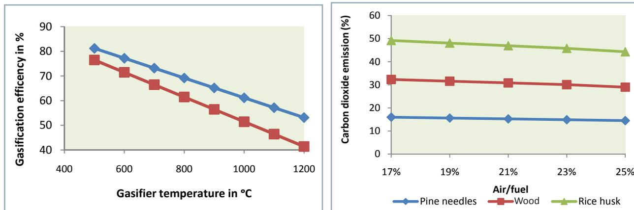
**Figure 6** a) Effect of gasifier temperature on gasification efficiency, (b) the variation of CO<sub>2</sub> emission with (air-fuel) A/F ratio
