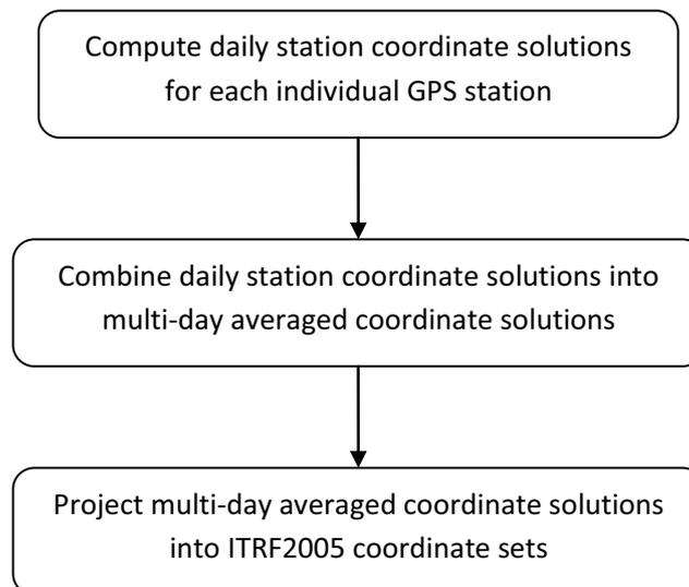
**Fig. 2.** PPP data processing steps (Satirapod et al., 2008).
