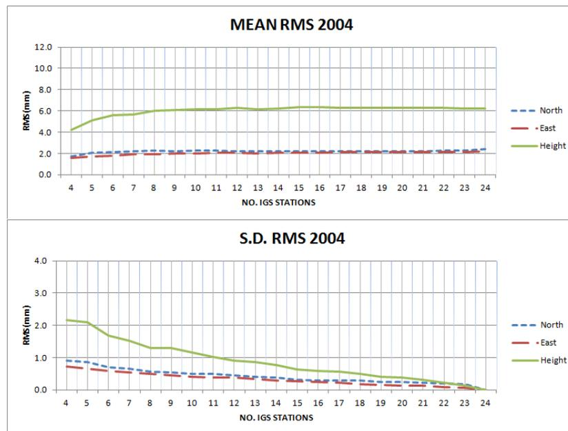
**Fig. 4.** Statistics obtained from varying number of IGS stations used in a mapping process for the 2004 campaign Top: Mean RMS values; Bottom: S.D. of RMS values.
