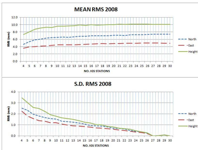
**Fig. 5.** Statistics obtained from varying number of IGS stations used in a mapping process for the 2008 campaign Top: Mean RMS values; Bottom: S.D. of RMS values.
