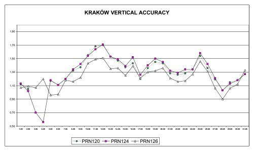
**Fig. 4.** Error of vertical coordinate observed in August 2010 with reference to the SBAS satellites (in [m]).
