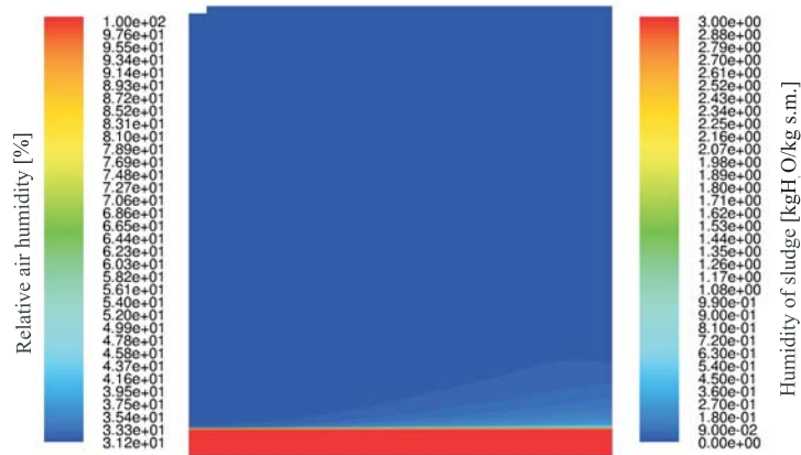
Figure 6. Distribution of humidity in the air and dried sludge for the modelled day; 13:00 hours.
