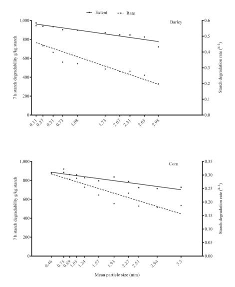
Figure 4. Extent and rate of 7 h *in vitro* starch degradation in the ground corn and barley with different mean particle size. Reproduced from Gallo et al. (2016)
