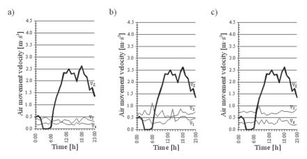
Figure 3. Wind velocity measurements  $(V_z)$  and air movement measurements  $(V_{1-6})$  in particular measurement points on 3 February 2012 inside the barn in Kobylany for three technological groups; a) group 1, b) group 2, c) group 3,  $V_z$ -wind velocity,  $V_{1-6}$ - air movement velocity (own source)
