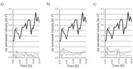
Figure 6. Wind velocity  $(V_z)$  and air movement velocity  $(V_{1-6})$  in particular measurement points on 7 February 2012 inside the barn in Kobylany for three technological groups; a) group 1, b) group 2, c) group 3 (own source)
