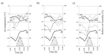
Figure 4. Temperature  $(\Theta_z, \Theta_{1-6})$ , relative air humidity  $(RH_z, RH_{1-6})$  and solar radiation intensity (I) on a cloudy day of 4 February 2012 inside the barn in Kobylany for three technological groups; a) group 1, b) group 2, c) group 3 (own source)
