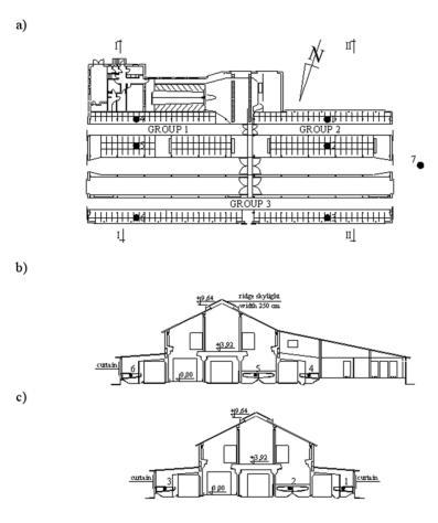
Figure 1. Location of measurement points: temperature, relative air humidity and air movement; a) horizontal projection, b) cross-section I–I, c) cross-section II–II, 1–7 – measurement points (own source)
