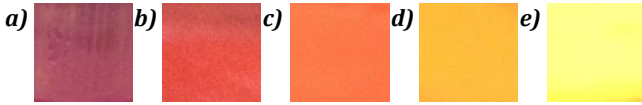
Fig. 6. Waspaloy heat colors in visible range of light: a) 550°C; b) 650°C; c) 750°C; d) 850°C; e) 950°C
