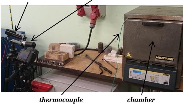
**Fig. 2. View of experimental set-up used in research**
