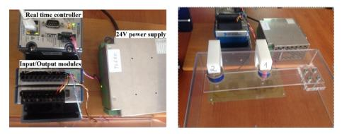
Fig. 2 Active vibration attenuation in a smart beam.
