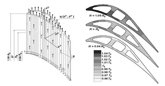
Fig. 6 Gas turbine blade: finite element model (left), and temperature distribution in blade fragment.
