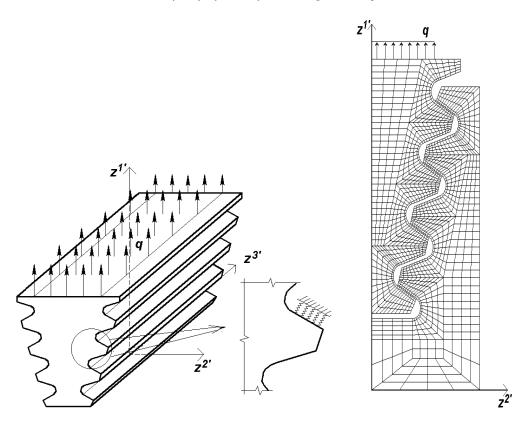
Fig. 4 Root of gas turbine blade: design scheme (left) and SFEM discrete model.
