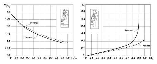
Fig. 5 Change in time of dimensionless stress intensity (left), and damage parameter.
