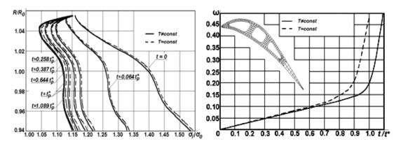
Fig. 7 Changing of stresses across the height of the blade (left), time-dependent damage parameter values.
