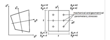
Fig. 1 Two-dimentional finite element in general (left) and local coordinate system.
