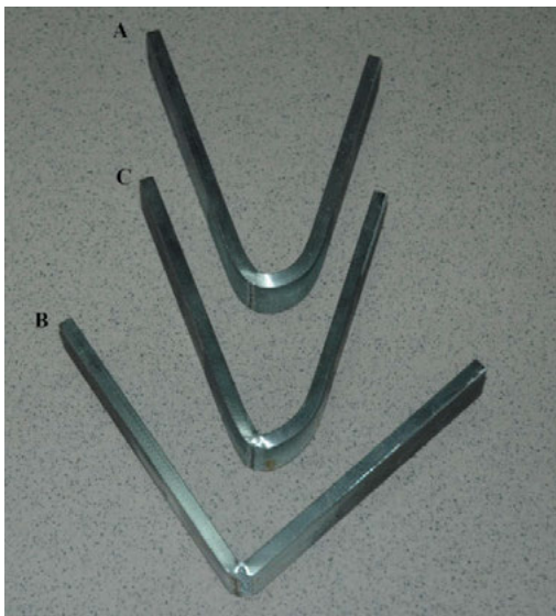
Fig. 9. A view of the samples after technological bend test (weld root bending) of 5.0 mm thick butt joints of S700MC steel sheets autogenous laser welded by the disk laser, evaluated according to the PN-EN 895 standard, Table 7
