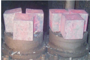
Fig. 11. Heating the tools by heated preforms
