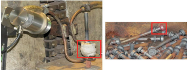
Fig. 7. Local induction heating of a forging
