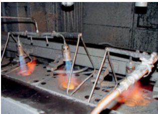
Fig. 13. Heating up the tools with gas burners
