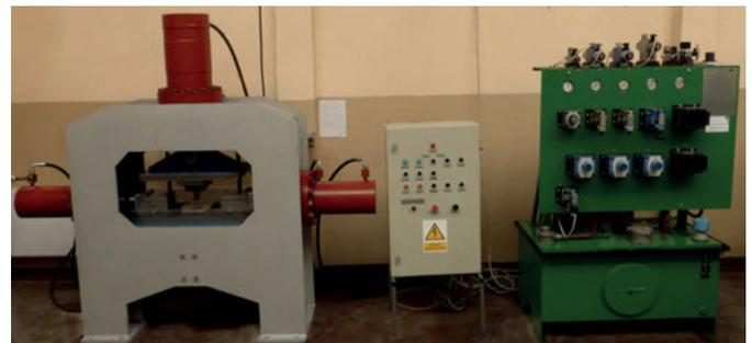
Fig. 4. Three-slide forging press
