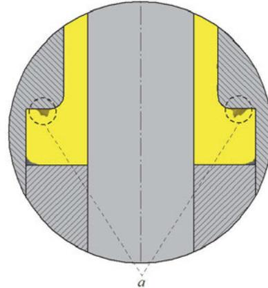
Fig. 3. Overlap produced in the second stage of flange extrusion
