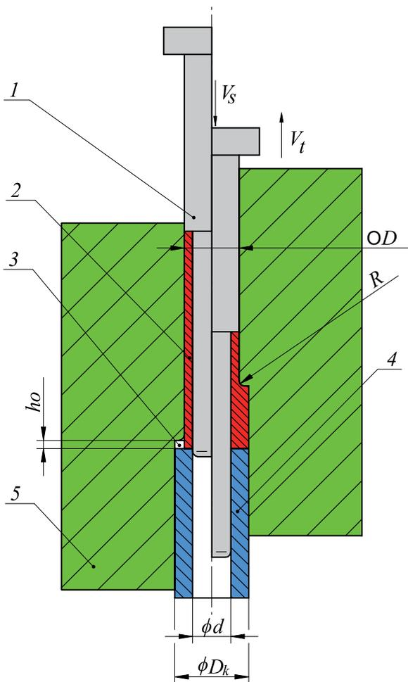
Fig. 1. Design of the device for extruding flanges: 1- punch, 2- workpiece, 3- space between the tools, 4- fixed sleeve, 5- movable sleeve,  $V_t$  – velocity of the movable sleeve,  $V_s$  – velocity of the punch,  $D$  – outside diameter of the workpiece,  $d$  – inside diameter of the workpiece,  $D_k$  – diameter of the flange,  $h_0$  – initial distance between the movable and fixed sleeves,  $R$  – edge radius of the movable sleeve
