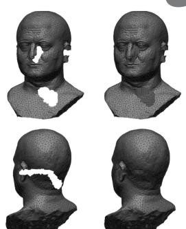
Fig. 7. Hole-filling example using the *PolyMender* software which generates a signed volume from the input mesh. The method presented by Ju (2004).
