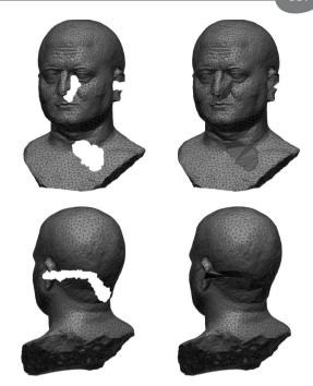
Fig. 1. Hole-filling example using the *Meshlab* software. Based on a variation of the method presented by Liepa (2003).
