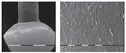
Fig. 3. SEM images of acrylic piercing (magnification X 30 и X 400)
