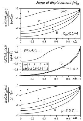
**Fig. 5.** Dependence of the form of displacement discontinuity on the relative remoteness of the force application point at the *p*-th step
