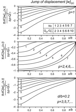
**Fig. 4.** Dependence of the form of displacement discontinuity on the magnitude of loading at the *p*-th step
