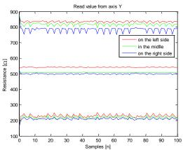
Fig. 6. The calibration of the touch panel in Y axis
