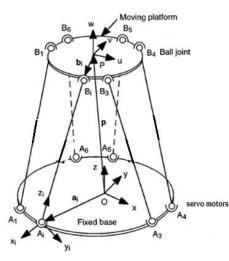
Fig. 1. Electrically actuated Stewart-Gough platform
