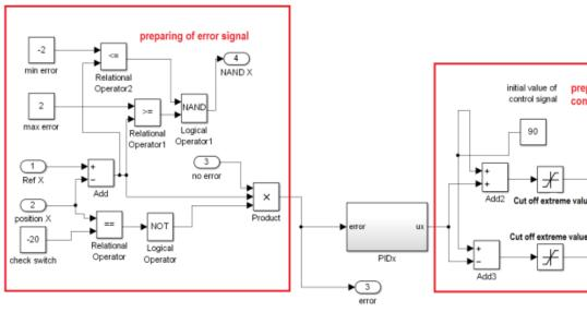
Fig. 9. The control scheme of the control of ball position's in X direction
