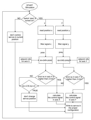
Fig. 4. Scheme algorithm of stabilization the ball on the platform  $(ref_x = 113 \text{ mm}, ref_y = 83 \text{ mm})$
