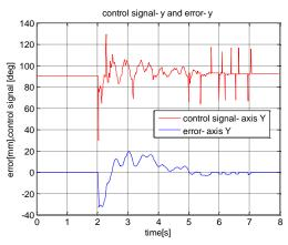
Fig. 11. The control signal and error signal derived by the PIDy controller
