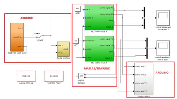
Fig. 3. The control scheme of the ball position
