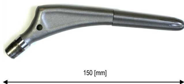
Fig. 1. General view of the fractured stainless steel stem
