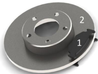
Fig. 1. Disc brake friction pair: 1 – brakepads 2 – corresponding brake disc
