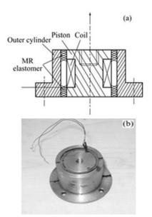
Fig.13. Schematic configuration (a) and photograph(b) of MRE absorber (Xiao et al., 2009)
