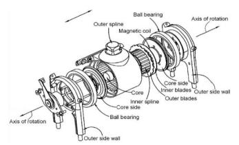
Fig. 10. A detailed exploded perspective view of a magnetorheologically actuated prosthetic knee (Thorarinsson, 2006)
