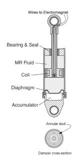
Fig. 3. Schematic of single ended MR damper and double ended MR damper, both produced by Lord (Spaggiari, 2013)
