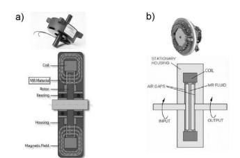
Fig. 9. Picture and schematic of a) MR based brake and b) clutch, both produced by Lord (Spaggiari, 2013)
