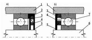
Fig. 8. Schematic of a sealing system in a motor bearing element with the use of MR fluids (Muc and Barski, 2007)
