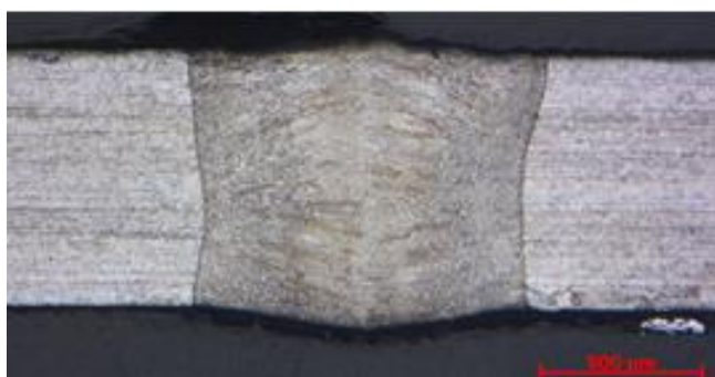
Fig. 12. Macrostructure of laser-beam welded AISI 304
